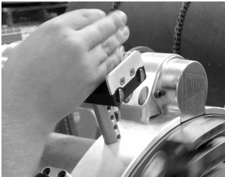
Figure 5-4. Push the trip knobs back to disengage the trips before starting the machine.
