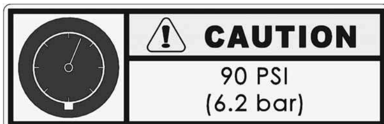
Figure 2-10. The air pressure label is attached to the air drive of pneumatic MDSF models. Do not operate the equipment with greater than 90 psi (6.2 bar) air pressure. (Part no. 90-401-02.)
