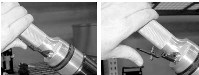
Figure 2-2. Hold the air motor trigger to operate the DynaPrep MDSF (left). When you release the trigger (right), the air motor shuts off.
