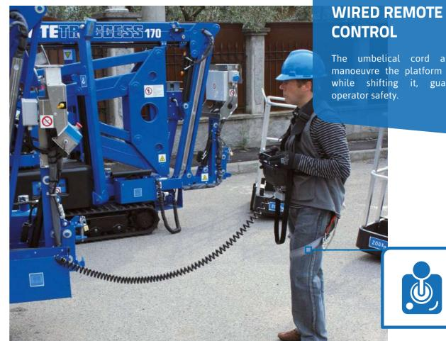
The umbelical cord allows to manoeuvre the platform smoothly while shifting it, guaranteeing operator safety.
