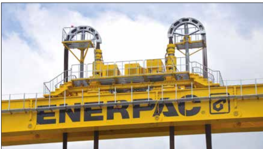
◀ HSL85007 Strand Jack System used on Enerpac custom Self Erecting Tower.
