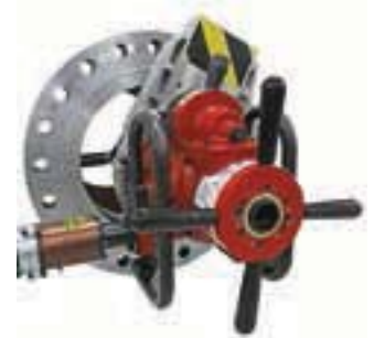
EP 424 Flange Facing with single point machine slide
