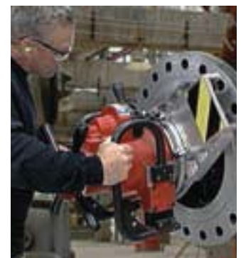
Faces flanges up to 36in (914 mm) with optional slide
