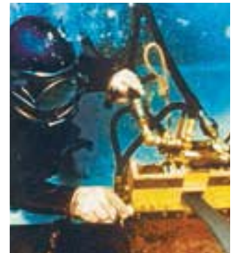
Model HE Hydraulic Trav-L-Cutter suitable for full immersion
